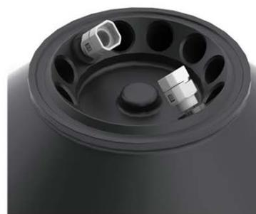
Balance centrifuge. Spin at 3000x g (RCF) for 30 seconds
