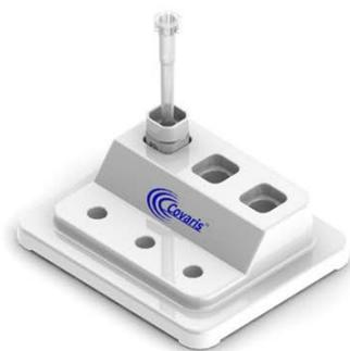
Carefully load sample through the septa making contact with the glass wall of the microTUBE
