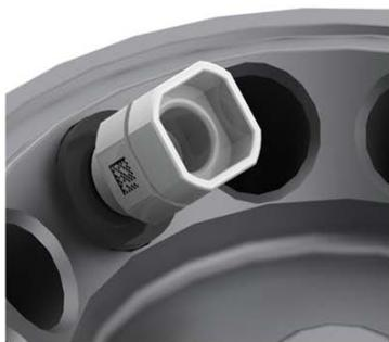
Load microTUBE-15 into the centrifuge using microTUBE Adapter (PN 500406)
